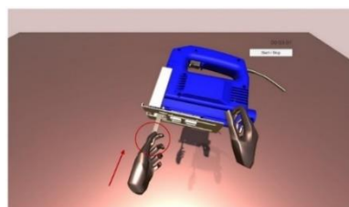
Fig. 6. The injury cause from trainees move their hands to hold the saw blade directly from the bottom of sharp side.
